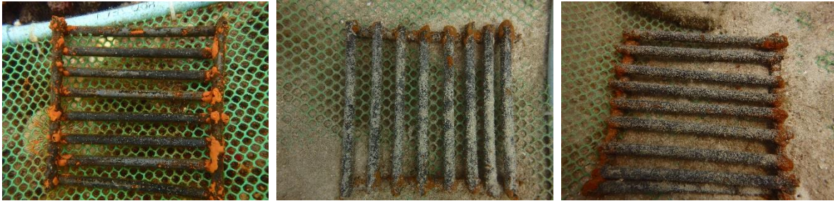
Figure 11. The three steel samples used for the substrate survey after two weeks of survey. All three steel samples showed sponge settlement on the sides and the edges.
