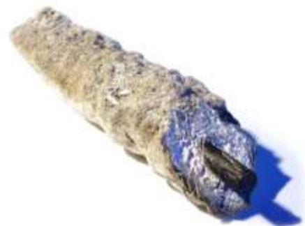
Picture 4.1 This picture shows the mineral layer on a bar of a working mineral accretion device after two years. Photo by Wolf Hilbertz.
